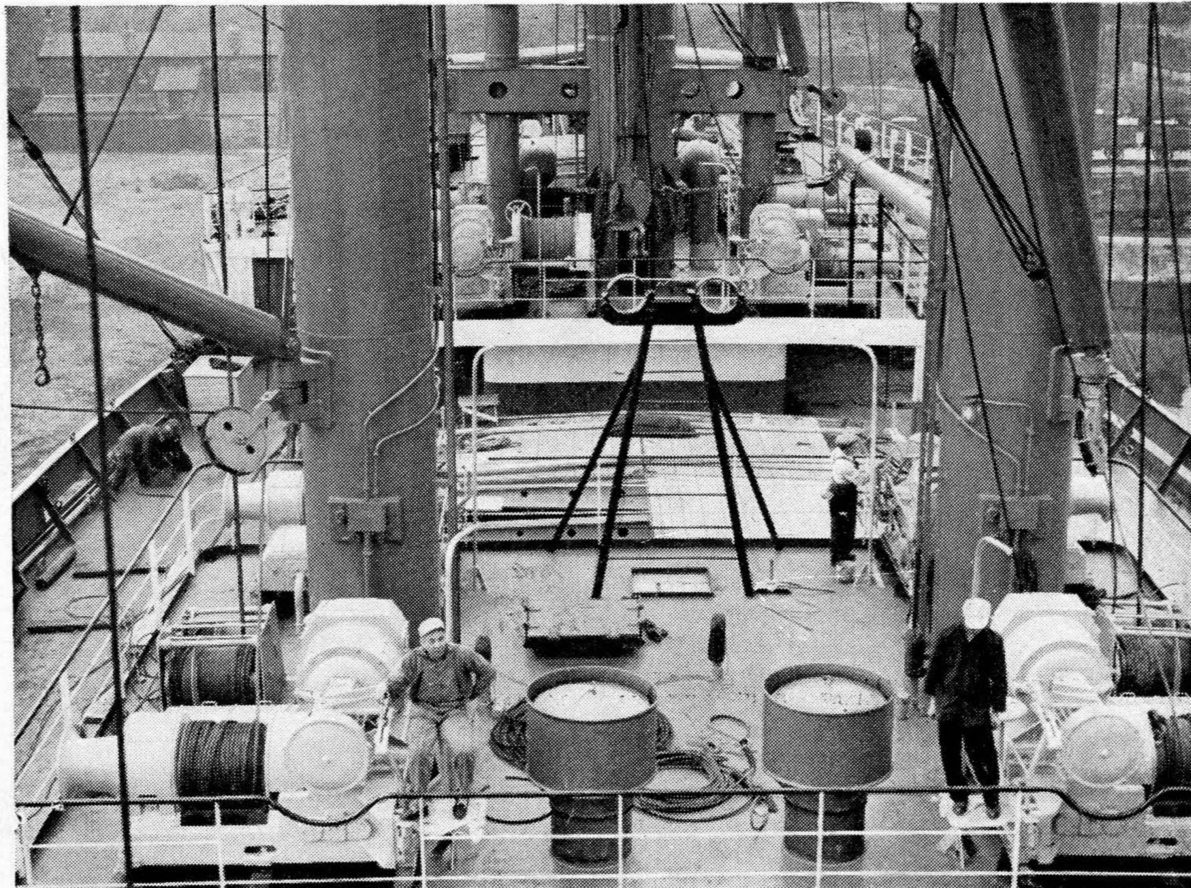
View of a winch deckhouse and the bridge from forward and (above) cargo-handling arrangements, looking forward.
